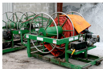
The AC Composter™ Covers are placed and removed using a Straddle Cover Winder. Push walls with man-doors protect the aeration system, allow easy access, and facilitate pile removal using front end loaders. The aeration hallway facilitates back to back zones. The main aeration plenum collects and delivers process air to the biofilter.
