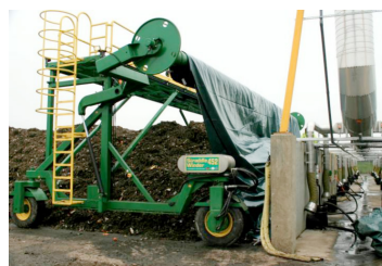
The AC Composter™ Covers are placed and removed using a Straddle Cover Winder. Push walls with man-doors protect the aeration system, allow easy access, and facilitate pile removal using front end loaders. The aeration hallway facilitates back to back zones. The main aeration plenum collects and delivers process air to the biofilter.
