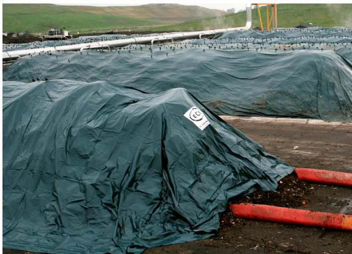
The CompDog™ is deployed and retrieved using Dog Rollers. The CompDogs are buried underneath the piles and later removed forming the aeration vault.
