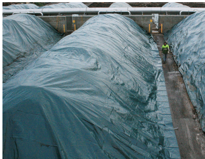
Full sized AC Composter™ zones can reach 550 mt 3 . The AC Composter Covers are placed and removed using a Straddle Cover Winder. Push walls protect the aeration system and facilitates pile removal using front end loaders. The aeration hallway allows back to back zones reducing footprint. The negative aeration system collects and delivers process air for scrubbing in a biofilter.
